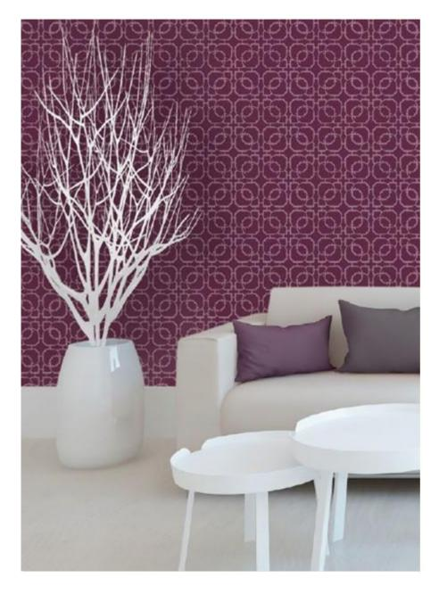
Vinyl based wallcovering on textile backing is a wallcovering using a woven textile base. The textile base (scrim) can be cotton or a polyester-cotton blend.
